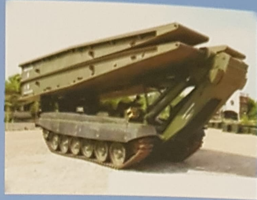
T 72 BRIDGE LAYERED TANK
